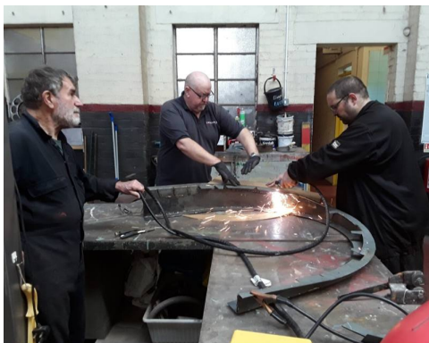
Ty, John and Chris use the plasma cutter to produce the various parts for 262's new front wings. [Keith Walker]
